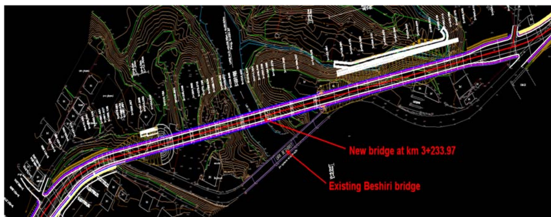
Figure 4: New bridge, and on the slightly corrected route
